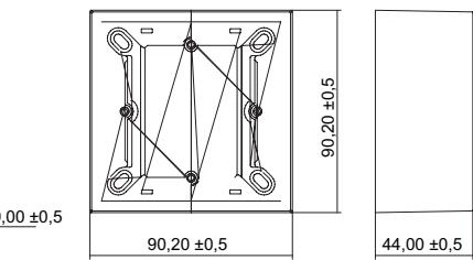
dimensions of single surface-mounted box, deco "H"element,
